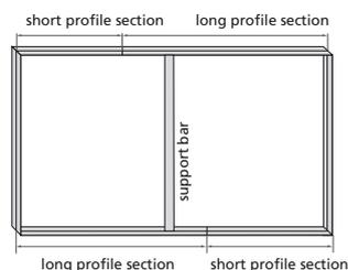
arrange short and long profile section staggered, mount support bar centred in the frame
