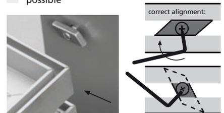
Position support bar(s) with widths from 4.81 m to 7.0 m:
